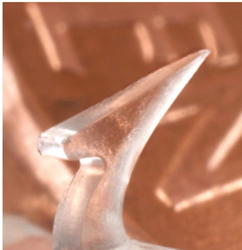
Bioresorbable tissue anchor with 0.00098" radius on end of barb
